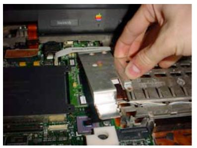
Lift the heat shield up and away from the network card.
