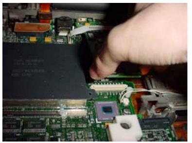
To remove the network card, grasp the card as shown. Lift the card up and towards you. It should easily come free from its connector.
