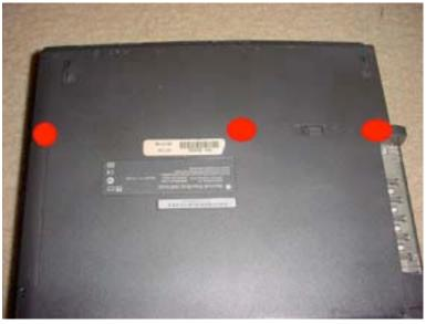
To remove the keyboard, start by flipping your unit over. Locate the 3 Torx T8 Screws as shown, and remove them.
