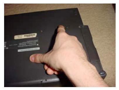
To remove the floppy or CD-ROM drive, start by flipping your unit over. Locate the lock switch as shown, and move the switch to the unlock position.
