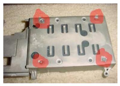
Remove the 4 Torx T8 screws from the location shown on the caddy.This will release the hard drive from the caddy.
