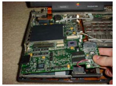
Grasp the logic board as shown. Pull the board out and to the right and up. Then pull the board towards you. You will need to work with the board a little bit to get it to come out.
