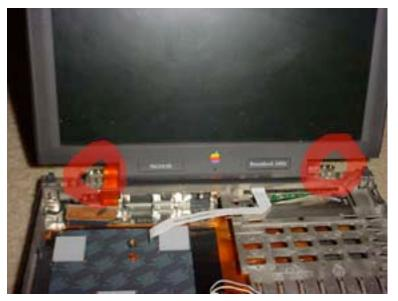
(You do not need to remove every component to remove the display. You need to follow every step up to and including the clutch cover removal. Then disconnect the orange display cable from the logic board and remove the two Torx T8 screws as shown.
