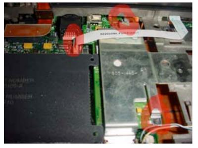
Heat Shield & Network Card Removal
