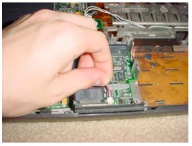
Disconnect the fan connector as shown.
