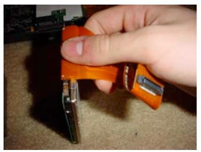
Remove the hard drive connector cable from the hard drive by pulling directly up on the cable. You must pull gently and directly up or you will bend the hard drive pins on the hard drive.
