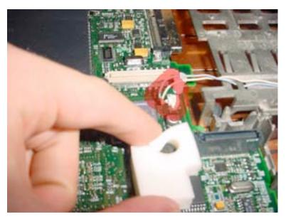
Remove the white airflow detector (white foam piece) from the logic board, and disconnect the LED indicator as shown.
