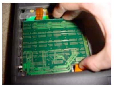
You will now have access to the ram. To remove the ram, simply grasp the chip as shown and pull up. The ram will easily come free from its connector.
