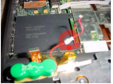
Flip the grill over, and you'll notice the speaker cable as shown. Disconnect the cables at the connector by simply pulling them apart. The speaker grill will then be free.
