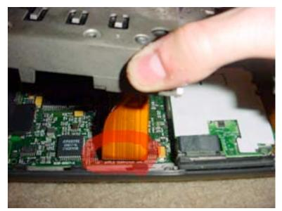
Next, lift up on the hard drive caddy, and this will reveal the hard drive connector cable as shown. Undo the hard drive connector cable, and this will free the caddy.
