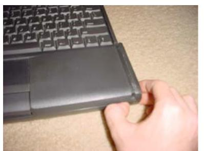
Begin all repairs by first unplugging your unit and removing the battery. To remove the battery, locate the eject mechanism on the front of your unit as shown. Push the button in and slide the battery out and to the right.
